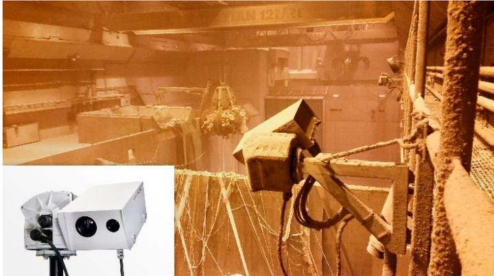
Fig. 2: The combination of pan/tilt heads, infrared cameras and visual cameras offers an excellent overview of the material located in the various stacking compartments.
