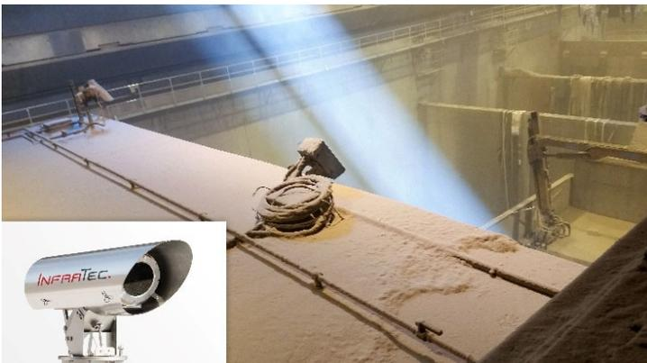
Fig. 1: Permanently installed infrared cameras are used for monitoring the hopper.
