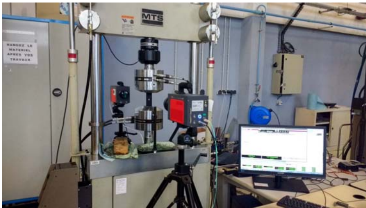
Figure 2: Experimental setup. The ImageIR® 8300 hp is on the left, the ImageIR® 10300 on the right and the specimen in between.
